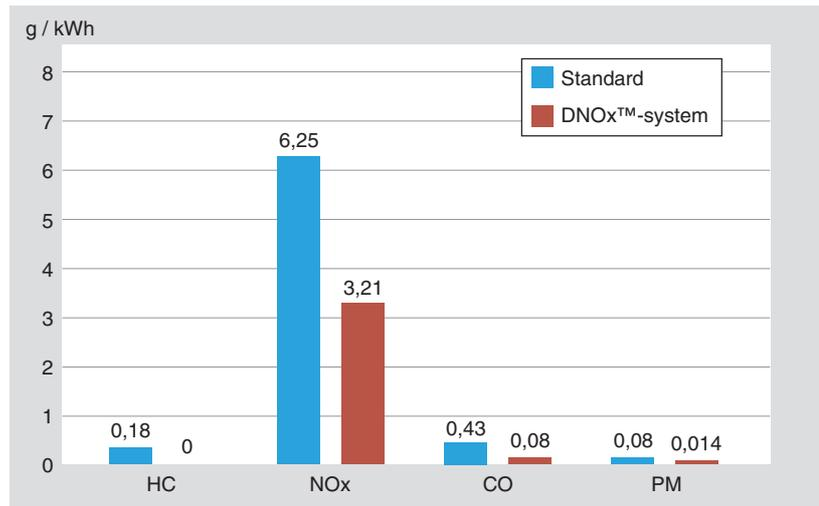
Figure 5 Results of bus tested according to simulated ECE R49 with a 10-litre bus engine of Euro 2-type
