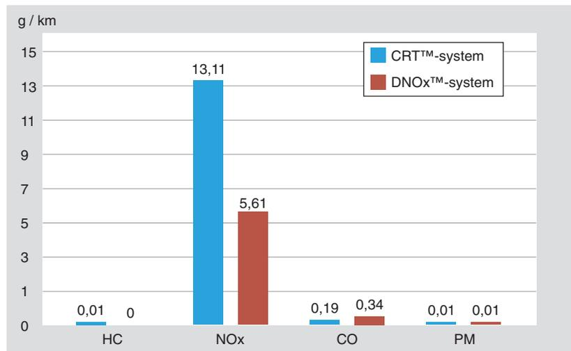
Figure 6 Results of bus tested according to the Braunschweig-cycle with a 10-litre bus engine of Euro 2-type
