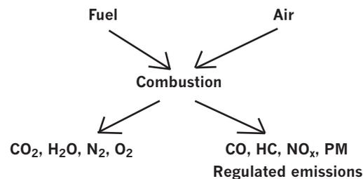
**Figure 1 Emissions from a diesel engine**
