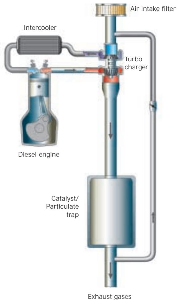
**EGR affects the formation of nitrogen monoxide during combustion**
